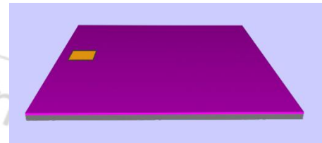
b) Deposition of the positive photoresist and UV exposure for mask 1
