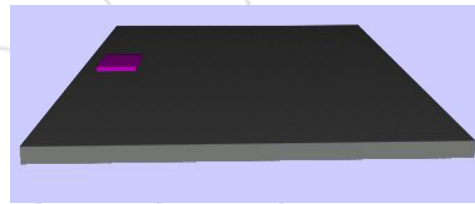
c) Etching to form the anchor part SiO 2
