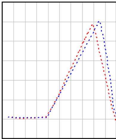
Figure 1.7: First mode shape of flexible four-bar mechanism for \theta_2=0^\circ .
