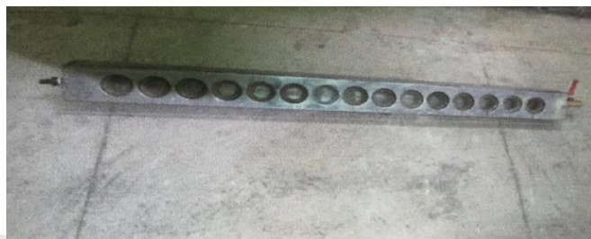
Figure 4: Header or heat exchanger
