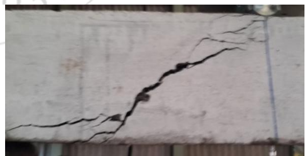
Figure 11: Failure pattern of L.B.1x8 beam
