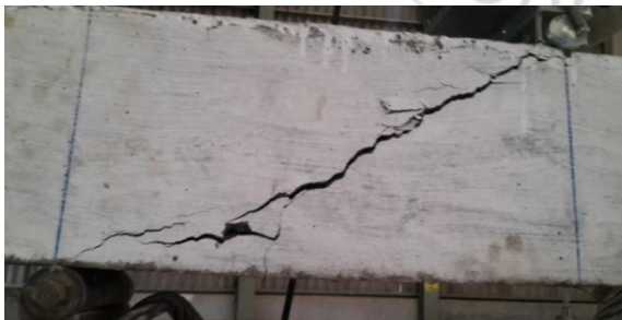
Figure 9: Failure pattern of L.B.1x6 beam
