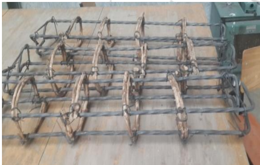
Figure 1: Fixed L.buchananii s shear reinforcements
