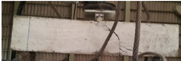
Figure 13: Failure pattern of L.B.2x10 beam
