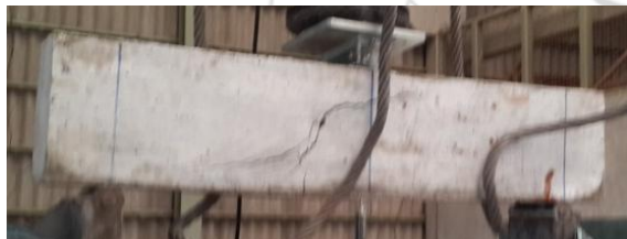
Figure 15: Failure pattern of L.B.2x13 beam
