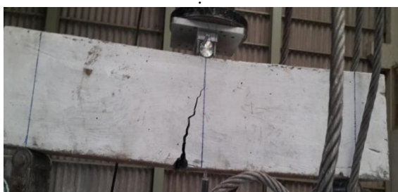
Figure 17: Failure pattern of Steel 1x6 beam
