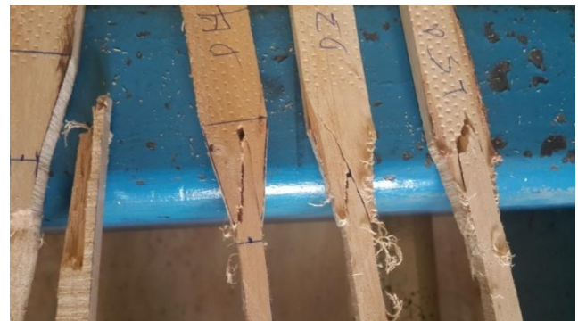
Figure 4: Mode of failure of tensile test samples
