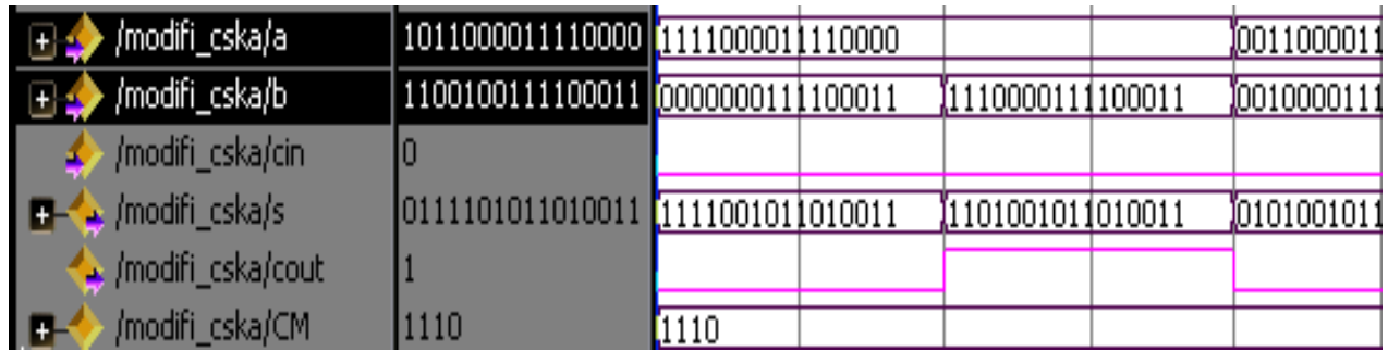
Figure 8: Waveform of Modified-CSKA
