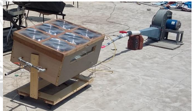
Figure 1: The Solar collector set up for Single and double pass
