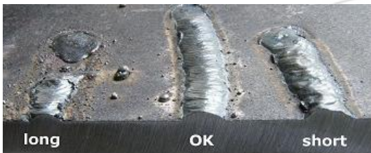
Figure 4: Arc length defects
