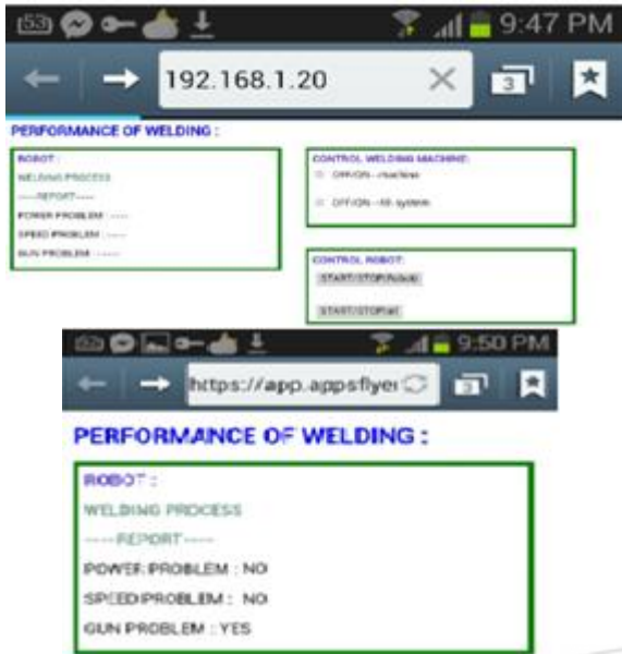
Figure 13: show result of Mobile SCADA
