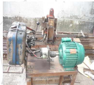
Figure 5: Assembly of Fuel pump cylinder & motor
