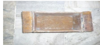
Figure 34: Punch for Bending
