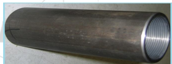
Figure 2: Internally threaded tube used as test section
