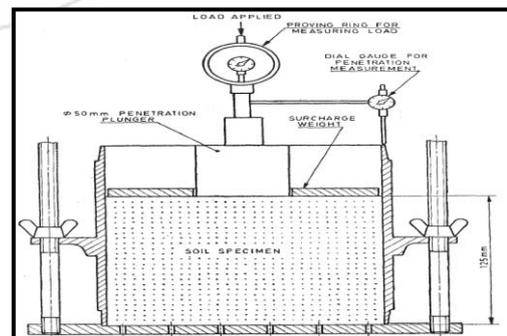
**Figure 3:** Set up for CBR Test
