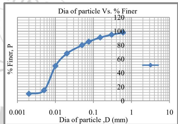
**Figure 2:** Particle size distribution curve (PSD) of Soil
