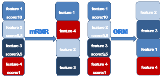
Figure 1: Illustration of mRMR (left) and GRM (right) mechanism. The first feature is correlated with the second and the third features, but the second and the third features are uncorrelated.
