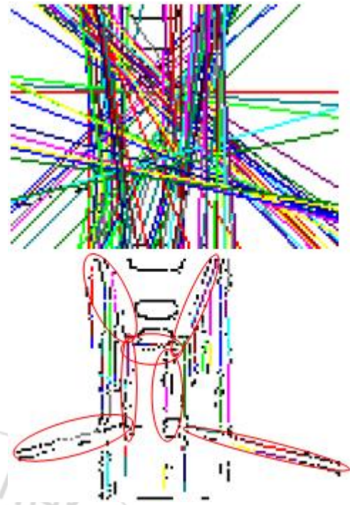
Figure 6: Lines and sub-lines found in image1 with T=300 (a) Lines found (b) Sub-lines found
