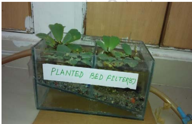
Figure 5: Planted bed filter used for treating the wastewater by phyto-remediation technique
