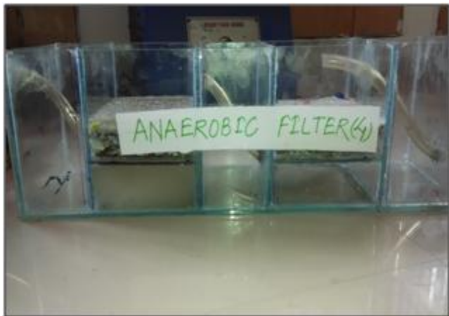
Figure 4: Anaerobic Filter with bagasse fly ash and sand
