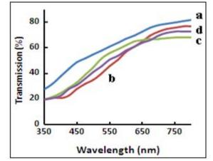
**Figure 1:** Transmission verses wavelength of as deposited thin films prepared at different substrate temperature a) 250°C b) 275°C c) 300°C and d) 325°C
