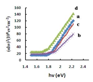
**Figure 2:** The graph between  $(\alpha h v)^2$  verses hv of as deposited thin films prepared at different substrate temperature a) 250°C b) 275°C c) 300°C and d) 325°C
