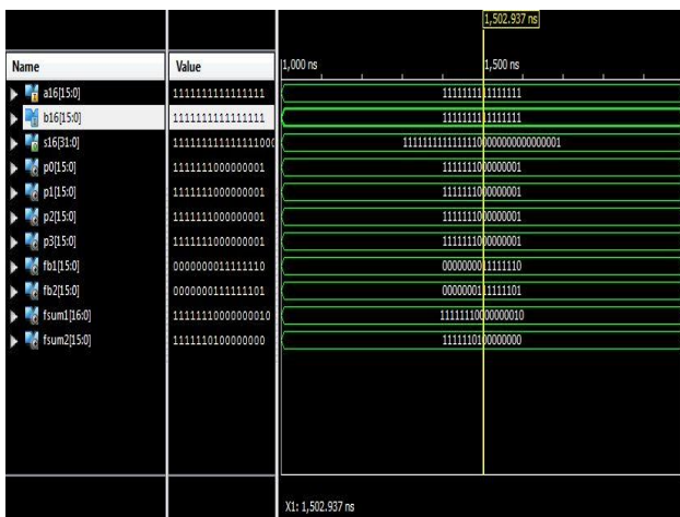
Figure 7: Simulation Result of 16X 16 bit Vedic multiplier using Brent Kung adder
