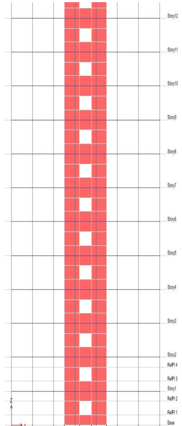
Figure 4: Elevation view showing shear wall openings of size 2 m X 1.2 m
