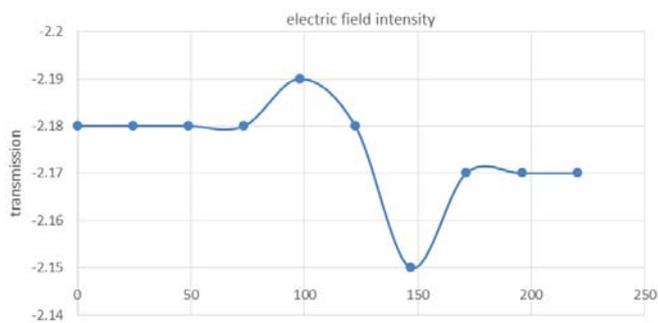
**Figure 9:** shows the relation between transmission and electric field intensity after infiltration with EBBA liquid crystal at 650 nm.
