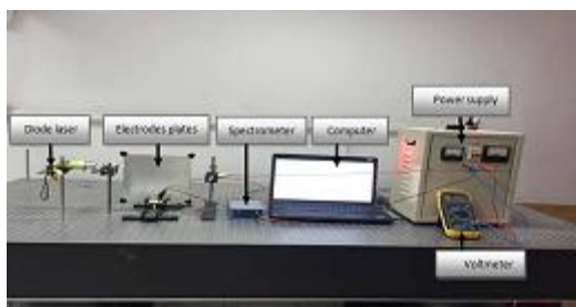
Figure 5: Photographs of electric field sensor setup.
