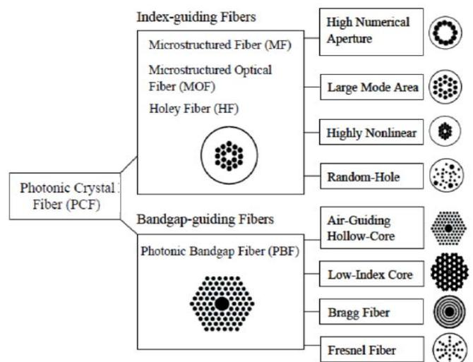
Figure 1: Categorization of photonic crystal fibers [5].
