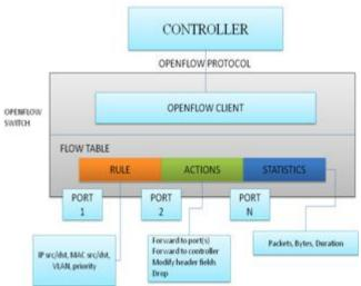
Figure2: The Open flow architecture
