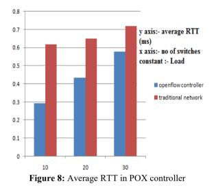
The above graph shows the average RTT in milliseconds in traditional network and Openflow network using POX controller. The average RTT in Openflow network in much less than the traditional network showing better performance in Open flow network.
