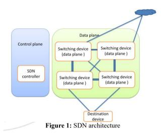
POX is a open source SDN controller and a platform which allows to program the devices through controller and for prototyping the network control software using python programming language. POX is mainly used for research purpose in the field of SDN. POX can run anywhere, particularly it targets Linux, MAC OS and windows.The POX contains reusable sample components for shortest path selection, controlling the switch behavior, etc. It also supports GUI and visualization tools.
