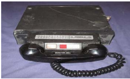
Figure 1: A mobile radio telephone [8].
