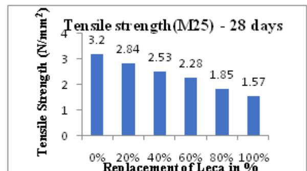
**Figure 5:** Split tensile strength comparison of L1 & L3
