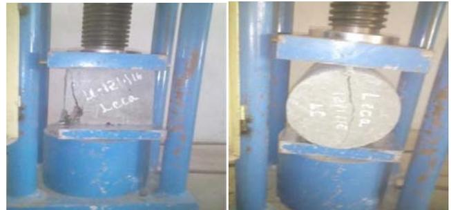
**Figure 3:** Testing of cube and cylinder specimens
