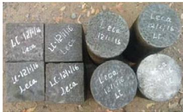
**Figure 2:** Cube and cylinder specimens
