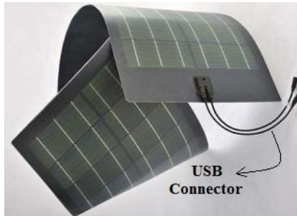
Figure 3(c): "Smart-Membrane" – Final Product (Source: Flexible CIGS solar cells - remodeled)
