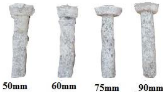
Homogenous soil Figure 5: Bulging of a stone column
