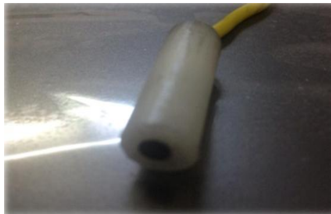
Picture 1: Handmade CPE modified by TiO 2 nanoparticles
