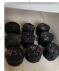
Figure 6: Marshall stability specimen
