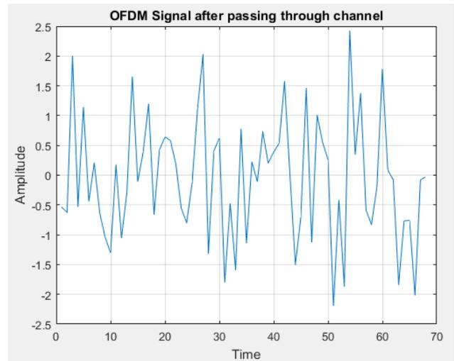
FFT is performed after passing through AWGN channel (as shown in 3.) and 2 bit IQ from Symbol de-mapper and this generates output bits (as shown in 4.)
