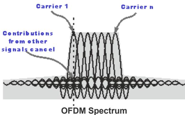
One requirement of the OFDM communication system is that it must be linear and any anomaly will cause interference between the carriers. This will introduce distortions that would affect the orthogonality of the transmission.
