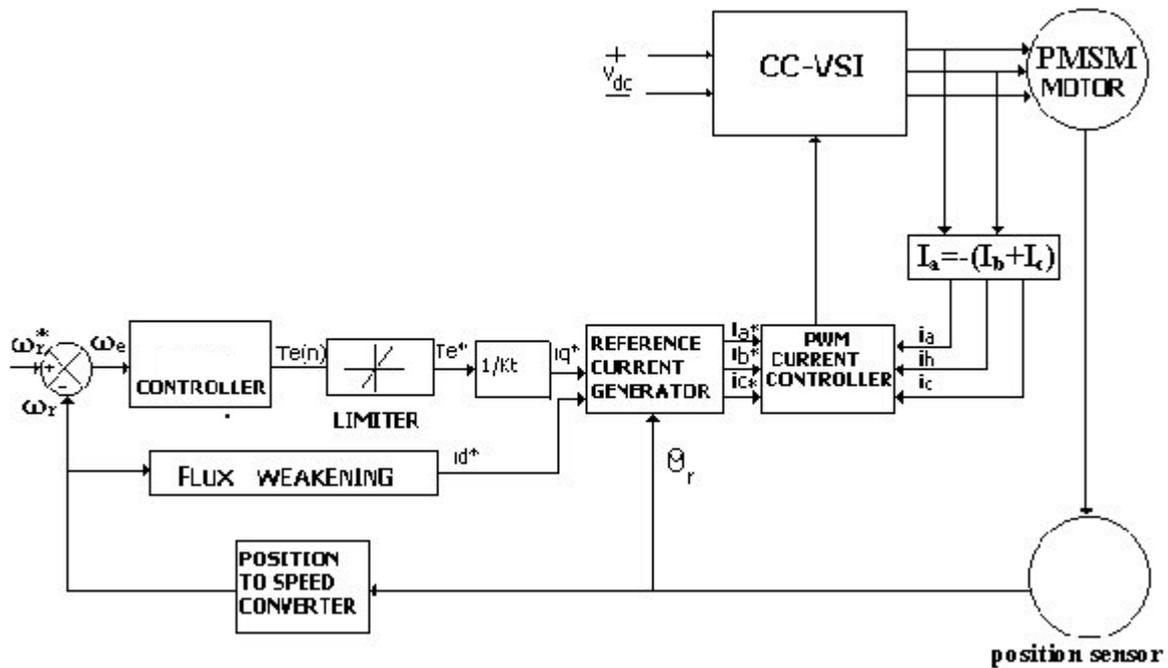
Figure 3: Schematic Block Diagram of PMSM Drive
