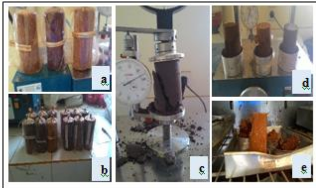
Figure 2: The stage of testing: a) the manufacture of the test object, b) curing process, c) testing of compressive strength (UCS test), d) weighing the specimen after testing, e) drying in an oven
