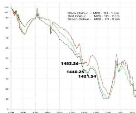
Figure 2: FT-IR graph for M20 grade of concrete (1D)
