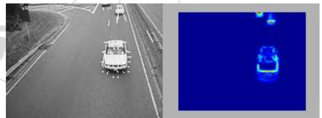
Figure 1.3: Optical flow estimation to obtain motion vectors (left) and pixel velocity magnitudes (right)[17].
