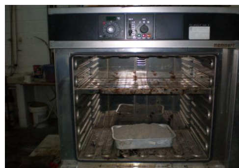
Figure 1: Fine Aggregate in the Oven
