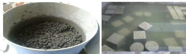
Figure 1: Concrete mixing Figure 2: Curing of Specimens
