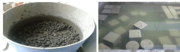
Figure 1: Concrete mixing Figure 2: Curing of Specimens
