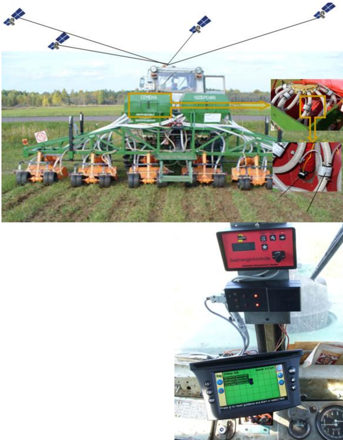
Figure 3: A new automated system to control Kombi band seeding of grasses and grass mixtures around grasslands and pastures with the use of global navigation and positioning.
