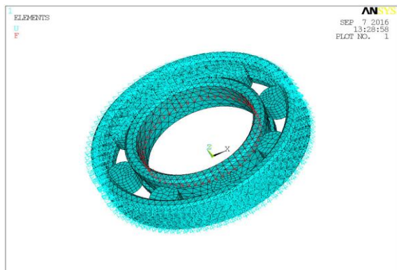
Figure 21: Boundary conditions applied to cylindrical bearing
