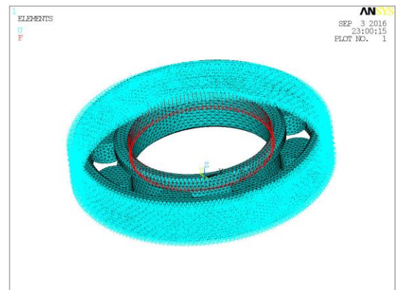
Figure 11: Applied boundary conditions of cylindrical bearing
