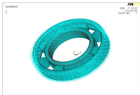
Figure 21: Boundary conditions applied to cylindrical bearing
