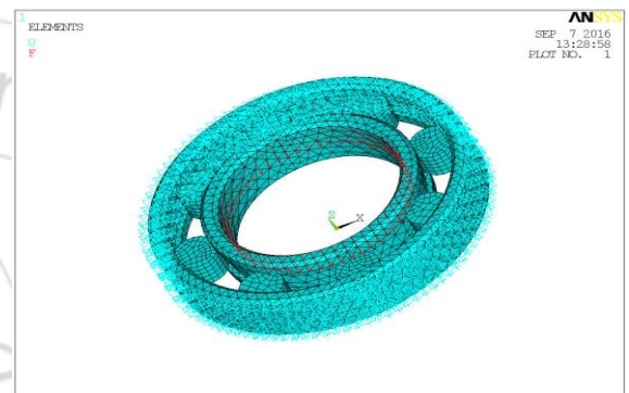
Figure 18: Boundary conditions applied to cylindrical bearing
