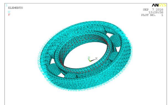
Figure 18: Boundary conditions applied to cylindrical bearing
