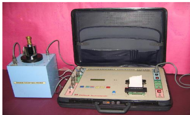
Figure 2: Emanometer and detector with lucas cell
