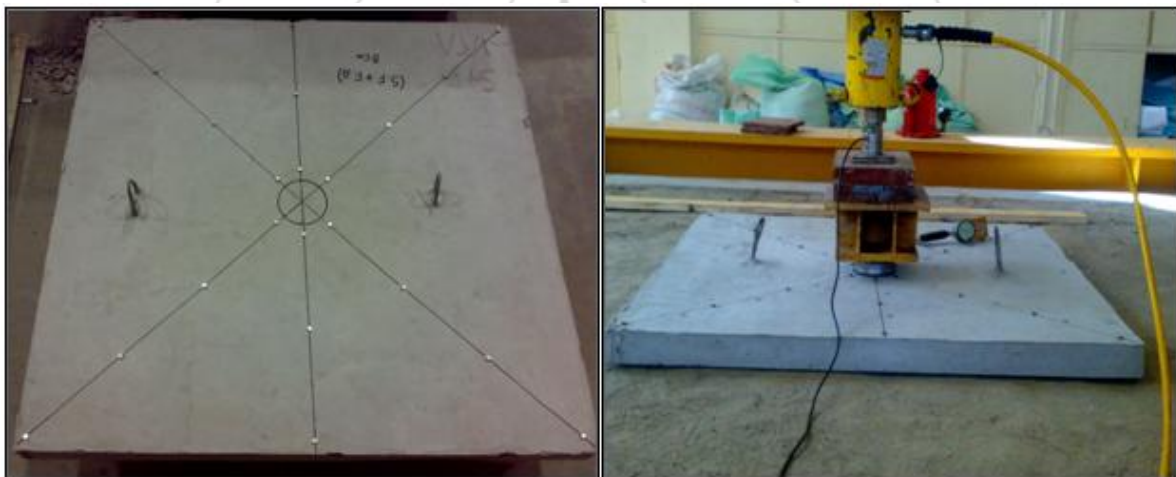
Photo 1: Measuring strain in slab
