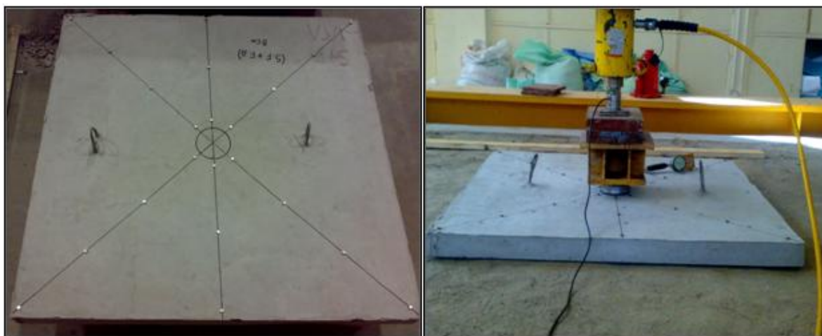
Photo 1: Measuring strain in slab
