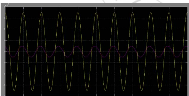
Figure 6: Vector group Phase Displacement for Dyn11 Transformer 4 before changes when transformer 1 is Dyn11 connected
