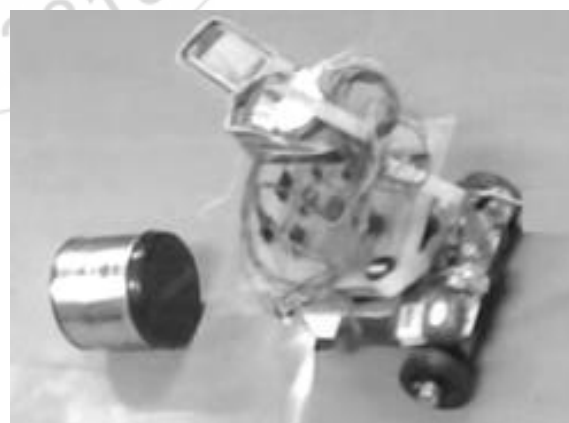
Figure 8(a): Detection of metal obstacle (cell phone activated)
