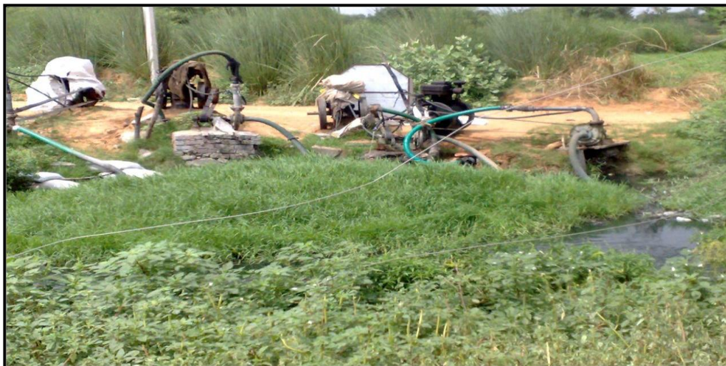
Figure 3: Series of pump sets, which is used to pump waste water for irrigating agricultural fields shown in the background.
