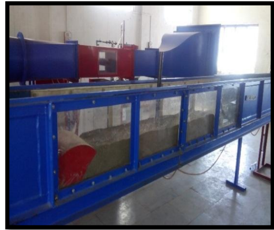
Figure 3: Tilting flume where experiment was conducted.
