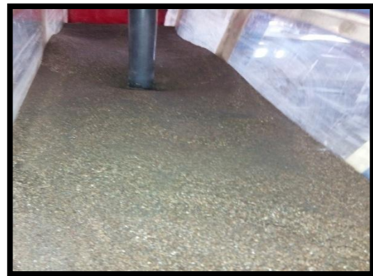
Figure 4: 25 mm pier with scour hole formation without splitter plate.
