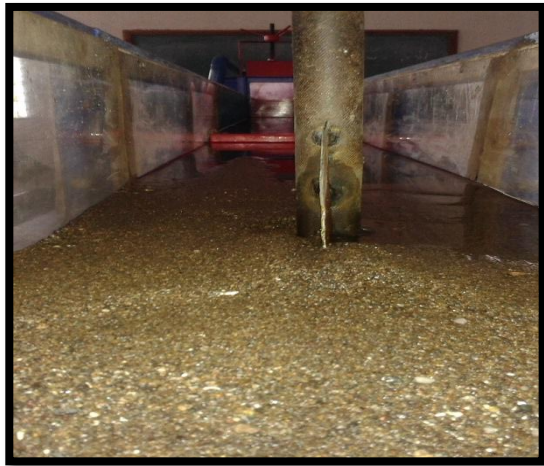
Figure 7: Splitter plate with pier assembly (25 mm dia.) is kept parallel to flow direction, due to which scour hole minimizes.
