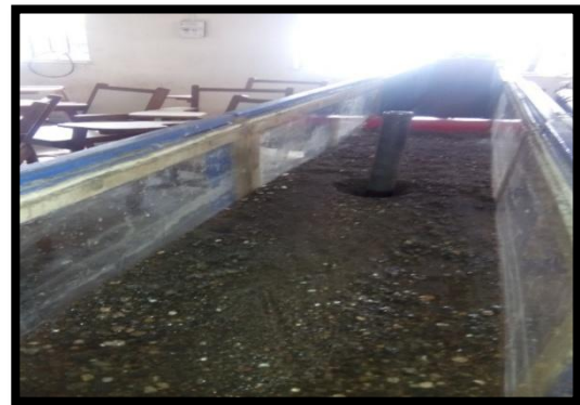
Figure 5: 50 mm pier with scour hole formation without splitter plate.
