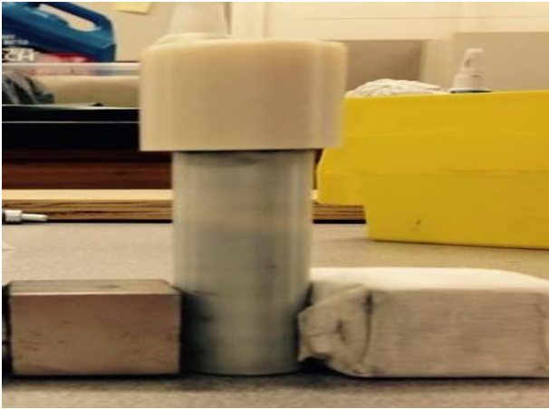
Figure 10: Applying magnetic field to the model using permanent magnets
