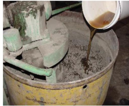
Figure 2: Pan Mixer Used for Manufacturing Geopolymer Concrete
