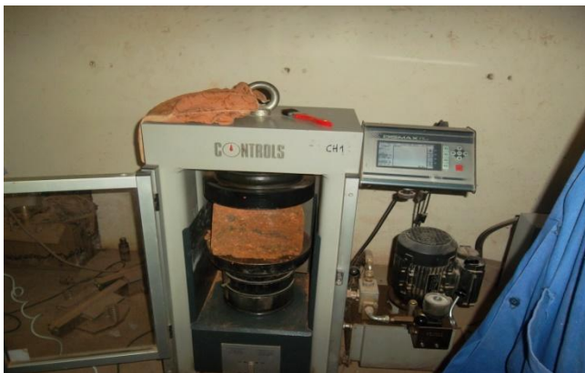
Figure 3: Blocks Placed in Compressive Strength Testing Machine for Crushing Test
