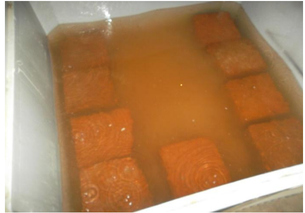
Figure 4: Blocks Placed in Water for Permeability Tests
