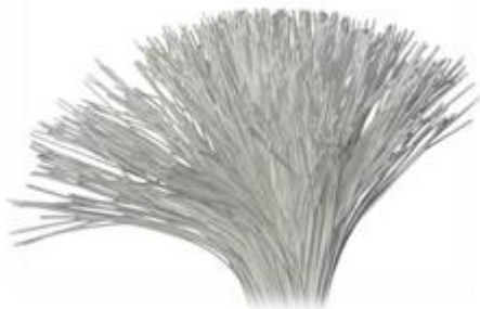
Figure 3: Bundles before potting
