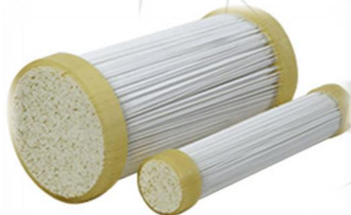
Figure 4: Bundles after potting
