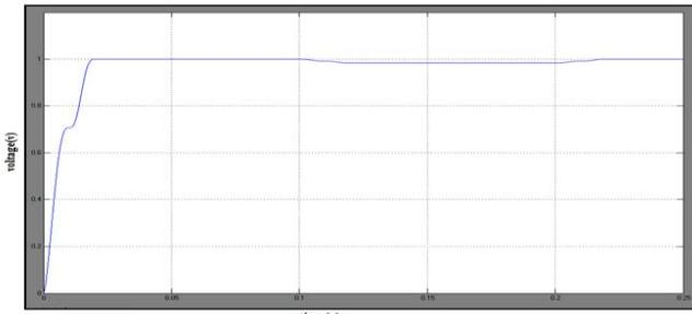
**Figure 4.2(c):** SLG voltage at load point is 0.983 p.u
