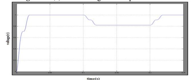
Figure 4.1(d): LL voltage at load point is 0.821
