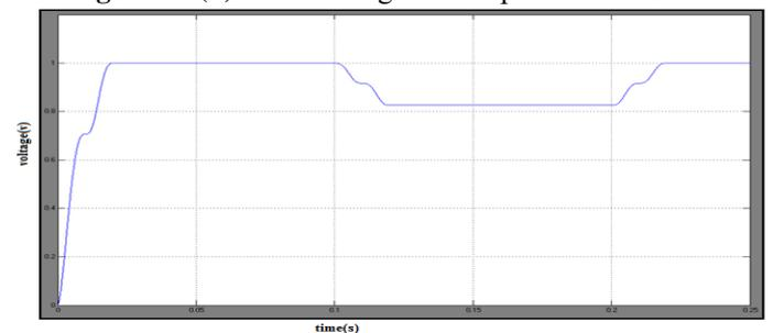
Figure 4.1(c): SLG voltage at load point is 0.825
