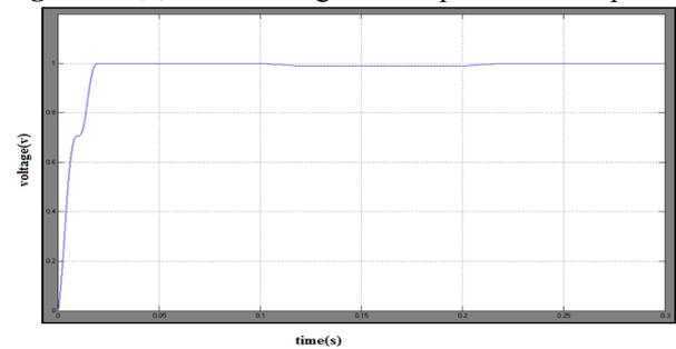
**Figure 4.3(c):** SLG voltage at load point is 0.997 p.u
