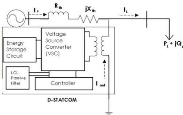
**Figure 2.1:** Schematic Representation of D-STATCOM
