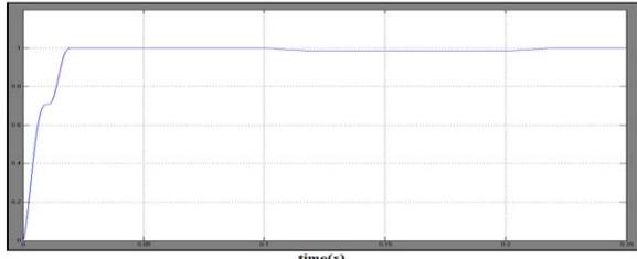
**Figure 4.2(b):** DLG voltage at load point is 0.985 p.u
