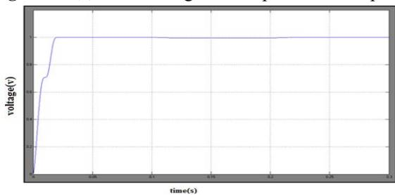
**Figure 4.3(b):** DLG voltage at load point is 0.995 p.u
