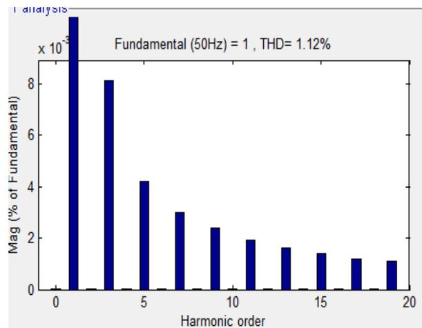
**Figure 4.4:** Harmonic spectrum of distortion output current with LCL passive filter with PI Controller.
