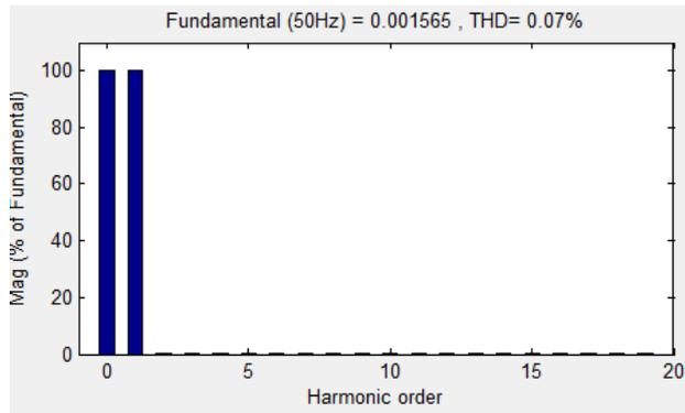
Figure 4.5: Harmonic spectrum of distortion output current with LCL passive filter with Fuzzy Controller.
