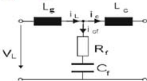
Figure 2.5: Circuit diagram for single phase LCL Passive Filter
