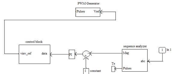
**Figure 2.2:** Block Diagram of Controller System
