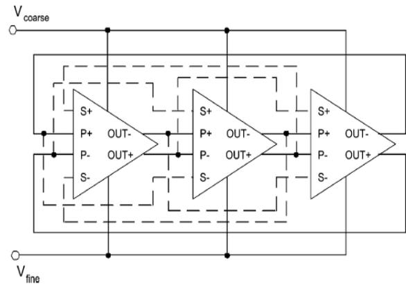
**Figure 3:** 3 Stage Multi Loop Ring Oscillator
