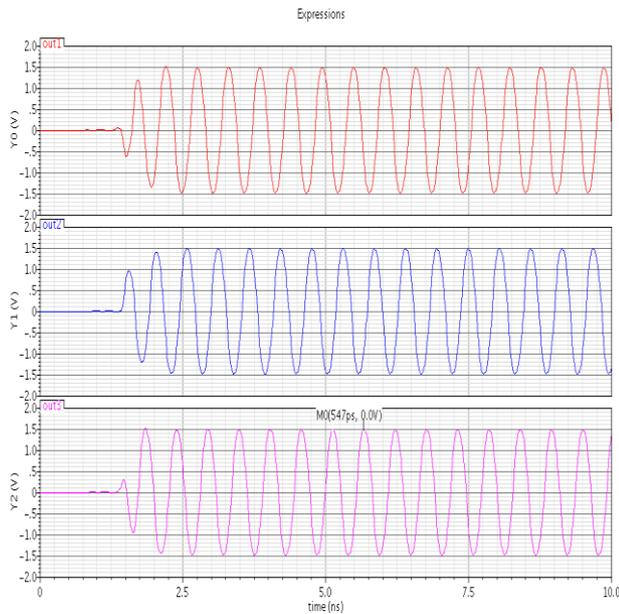
**Figure 4:** Transient Response of the Ring Oscillator
