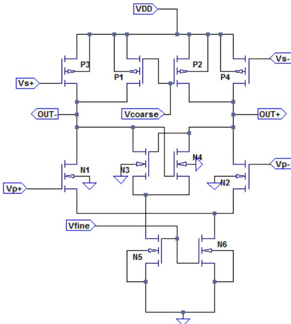
**Figure 2:** Proposed Delay Cell
