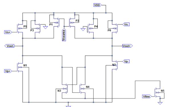
Figure 1: Conventional Delay Cell
