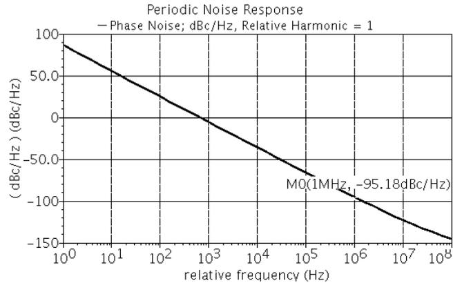
**Figure 6:** Phase noise of 2.1GHz center Frequency at an offset of 1MHz
