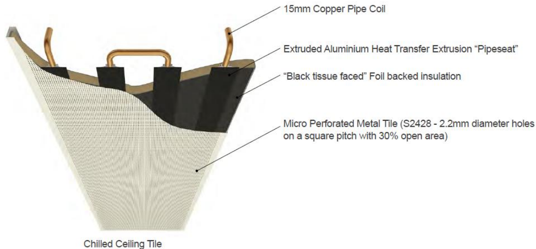
Figure 1.3: Chilled Ceiling Structure
