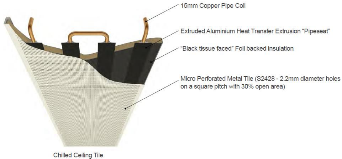
Figure 1.3: Chilled Ceiling Structure
