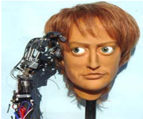
Figure 3: An android head and a robotic hand that are serving as biomimetic platforms for the development of artificial muscles.
