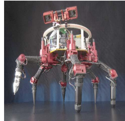
Figure 4: A new class of multi-limbed robots called LEMUR (Limbed Excursion Mobile Utility Robot) is under development at JPL
