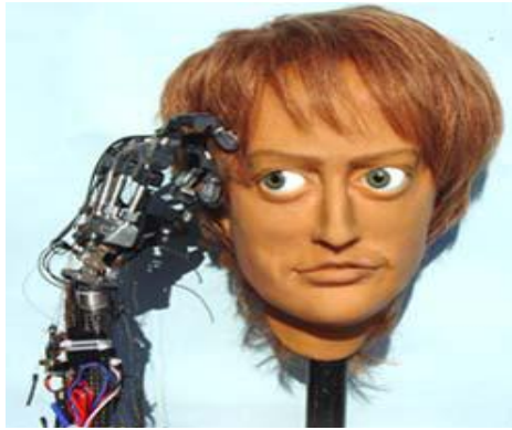
Figure 3: An android head and a robotic hand that are serving as biomimetic platforms for the development of artificial muscles.
