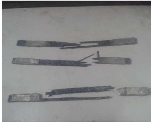
Figure 2 b. Test specimens. Figure 2: Tension test on FRP coupons.
