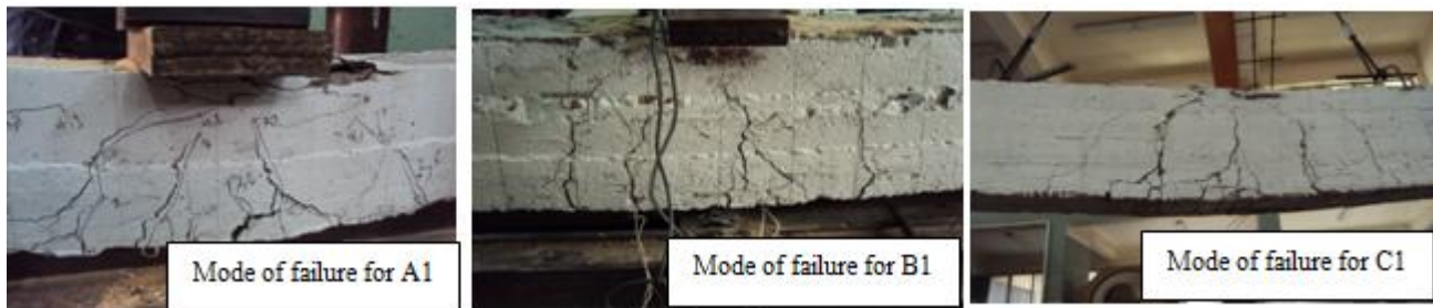
Figure 5: Mode of failure of control beams (A1, B1 and C1).
