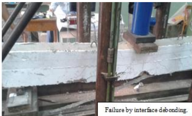
Figure 8 a: Mode of failure for beam A2.
