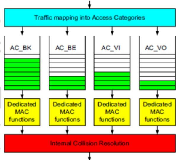
Figure 1: EDCA Functional Block Diagram
