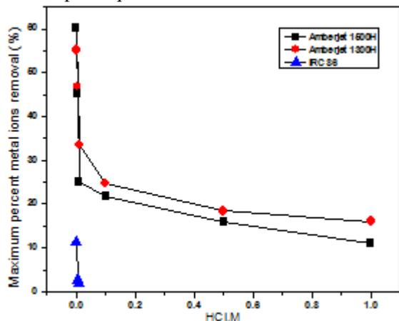
Fig.2. Effect of solution acidity on the cobalt removal by the resins
