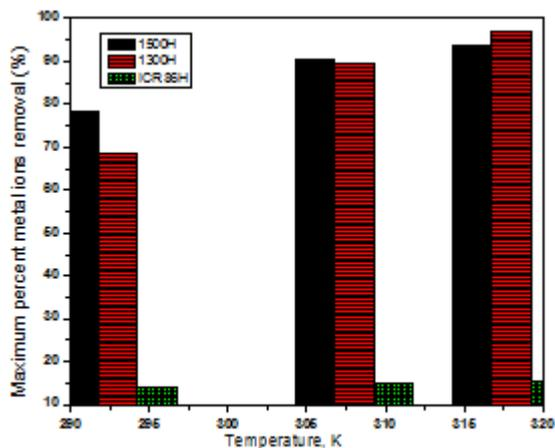
Fig.4. Effect of solution temperatures on the cobalt removal
