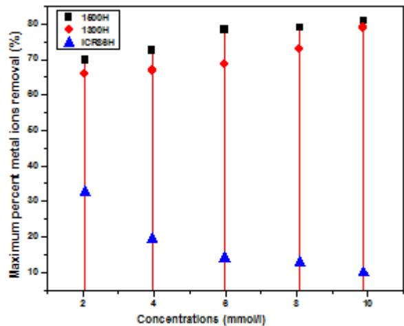
Fig.3. Effect of initial concentrations on removal of cobalt ions
